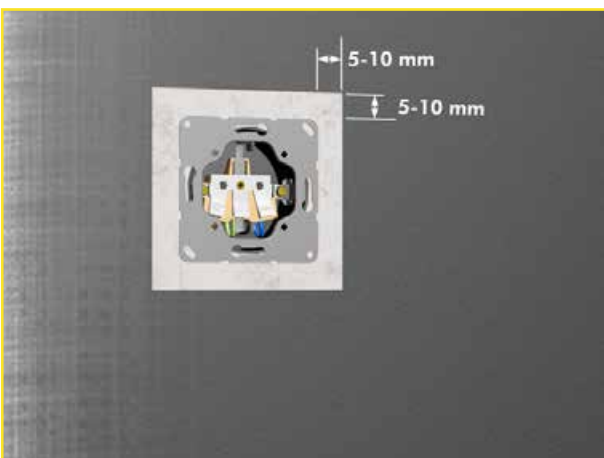
Fig.6: Keep about 5-10 mm distance to sockets and switching elements.
